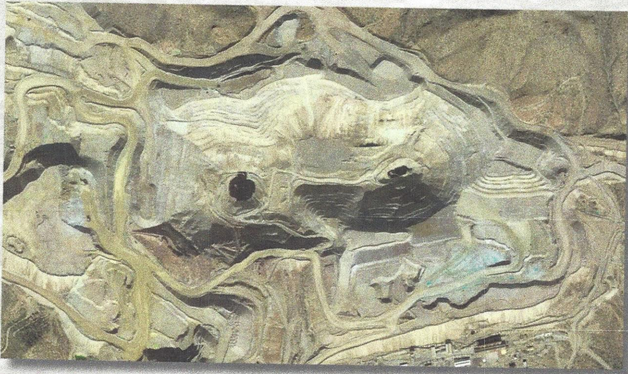
In-place leaching of rubblized and terraced walls of the Oxide pit at the Silver Bell mine, Pima County, Arizona (Satellite Photo from Google Earth - 12/20/2014)
